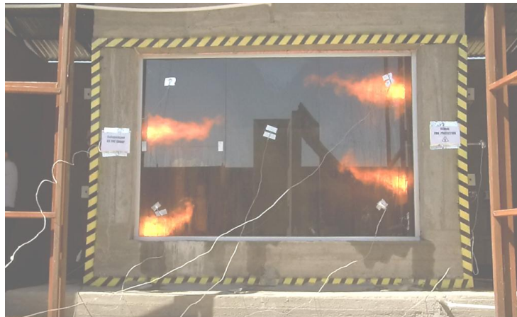
Figure 4 – Fragment of test to determine the actual fire resistance limit of glass under the real fire load
