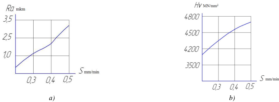
a - the effect of feed on the roughness; b - the effect of feed on hardness Figure 8 – Influence on the hardness and roughness of the cutting surface, Du=380mm; n=3500 rpm
