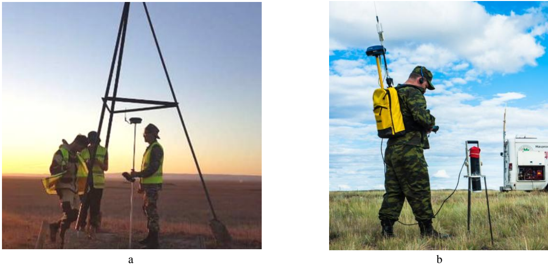
Figure 5 – Coordinates determination of points (a) and boreholes (b) by GPS technology
